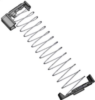
2. Insert follower into magazine tube and compress spring by pushing insert into magazine tube.
