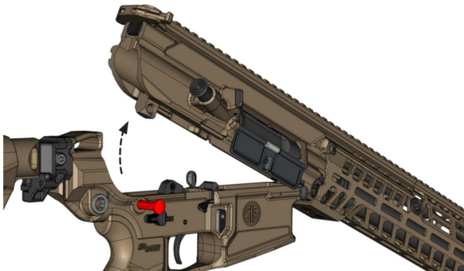
4. Push pivot pin from left to right until stopped by detent.
